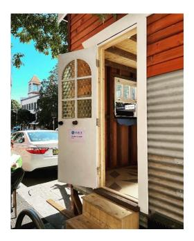
It's a compact, architect designed house. Built on a new 3 tonne trailer, made with a recycled Oregon timber frame, beautifully fitted with salvaged doors and windows and clad in reclaimed timber and corrugated iron.
